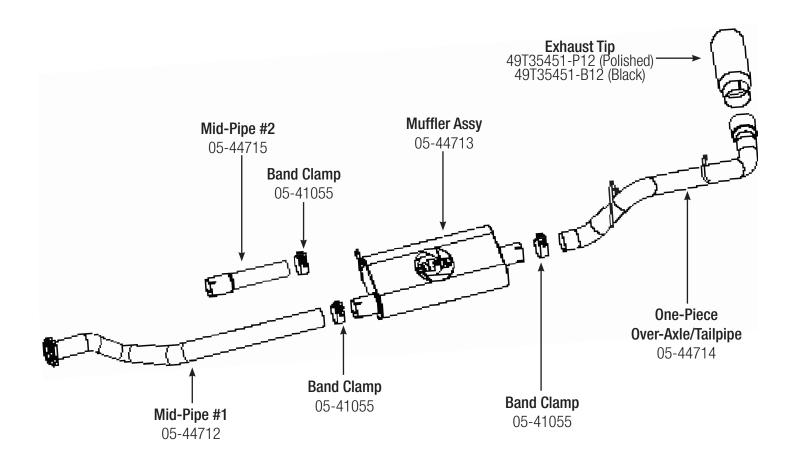
**Step 1: (Read Instructions prior to installation)** Remove your stock exhaust up to the catalytic converter from the rear of your truck working your way forward. Take caution not to damage the factory hardware and isolation mounts as they will be reused.
