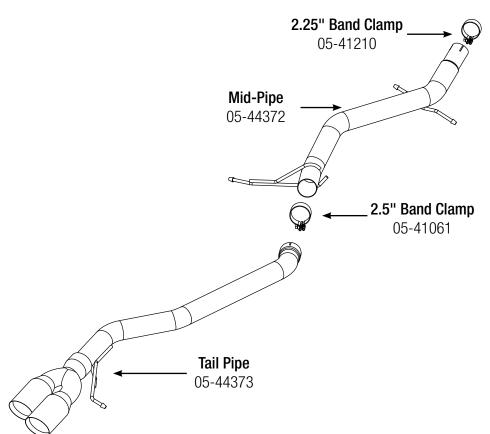
Step 1: (Read Instructions prior to installation) Remove your stock exhaust from the rear of your vehicle working your way forward. It will be necessary to cut the pipe to clear the rear axle. Do not cut the pipe after the cat; you will be using this slip connection. It is recommended to not fully tighten the clamps until the entire system has been installed.
