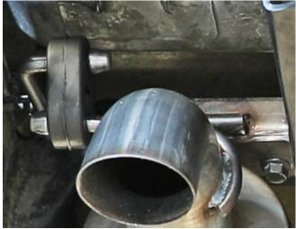
• aFe recommends that the tailpipe be at least 1/2"-1" away from any body panels to avoid heat related body damage. Tighten and secure.
