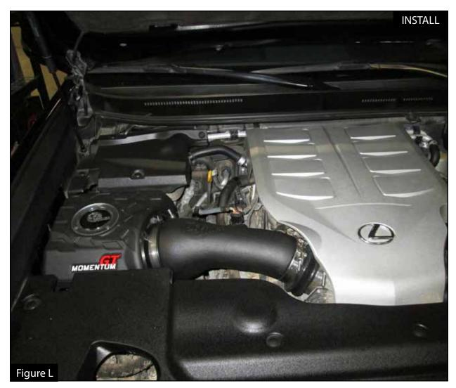
Refer to Figure L for Step 15 Step 15: Reinstall the engine cover.
