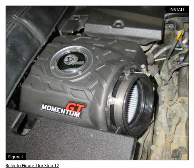
Step 12: Install the aFe POWER air filter and clamp into the airbox in the vehicle.
