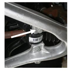
8. Using a **15mm** socket remove the 2 bolts from the lower shock mount.
