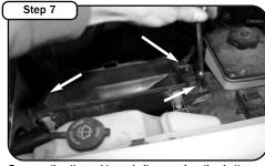
Remove the three 11mm bolts securing the bottom air box.Remove air box assembly.
