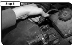
Remove the factory air temp sensor. Set aside for re-instal-
