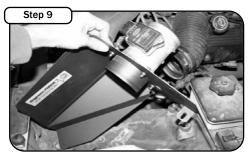
Reinstall new housing with MAF sensor connected.
