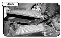
Remove upper air box cover and set aside for removal of MAF sensor. Remove factory air filter from bottom portion of cover.
