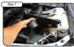
Install intake into vehicle. Position housing to tab.
