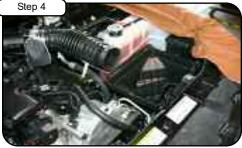
Loosen and remove OE intake tube with 5/16" nut driver. Remove bottom air box out of vehicle. Remove air temp
