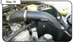
Insert tube in coupler. Place isolation mount in hole of housing.
