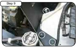
Secure housing using the 2 bolts and 1 nut from step 5 and tighten using 12mm socket or wrench.
