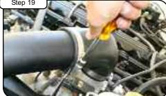
Tighten all clamps using 5/16" nut driver.
