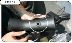
Install grommet in new intake tube.
