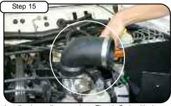
Install reducer elbow coupler to Throttle Body with clamps provided. Do not tighten. Turn page over and continue to page 2
