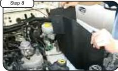
Place housing in vehicle and position holes of housing in factory positions.
