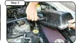
Unclip upper half of air box and pull back crankcase line.
