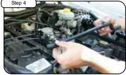
Remove crankcase line from valve cover.
