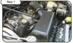
Complete Stock Intake. Disconnect battery before install.
