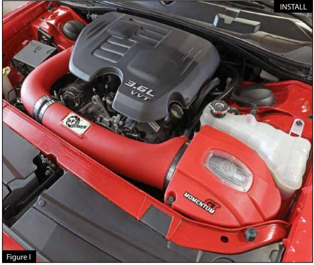
Refer to Figure I for Step 26 Step 26: Reinstall the engine cover. Page left blank intentionally
