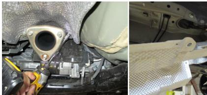
8. Once heat shield is removes from vehicle, disconnect the steering sensor connection. Disconnect steering rack connection on the side of the frame also.
