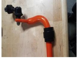
3. Install grease fitting onto supplied brackets. and install onto bar, using factory hardware.
