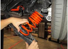
2. Using a screw, or floor jack, raise the lower control arm into position, and align control arm to the upright.
