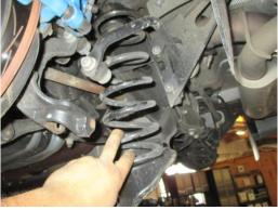
Rear aFe Coil Spring Installation
