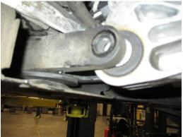
12. Re-secure the heat shield, and reinstall the exhaust
