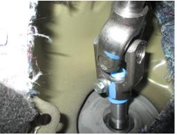
4. Use a 10mm socket to remove steering column bolt. **Before pulling the knuckle apart use a paint pen to mark the orientation of the two parts for proper column alignment later.**
