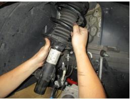
Front aFe Control Coil Spring Installation
