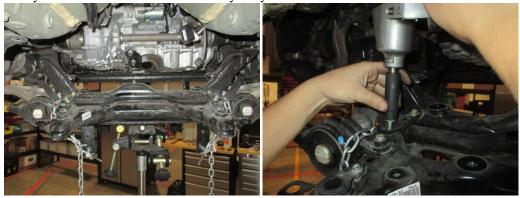
17. Before removing the brackets, take time to note the orientation of the OEM brackets.
