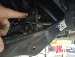
4. Remove the driver and passenger side sway bar mounts
