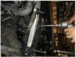
8. Reinstall the rear main subframe brace.
