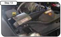
Place enclosed CARB EO sticker on a clean/smooth surface or or near the device. EO identification label is required in passing the Smog Check Inspection. Your installation is now complete. Please check all bolts and clamps perodically. Re-tighten if necessary. Thank you for choosing aFe!
