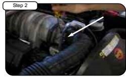
With 5/16" nut driver loosen the clamp on throttle body
