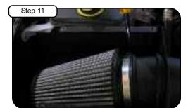
Re-connect air temp sensor harness. Install air filter and tighten using 5/16" nut driver
