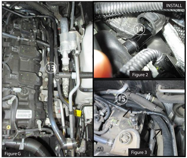
Step 16: Follow the factory crankcase hose to the rear of the engine 13.
