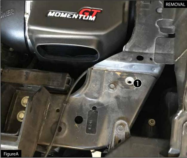
$\frac{\text{Refer to Figure A for Step 1}}{\text{Step 1: Remove the OE bolt 1}}.$
