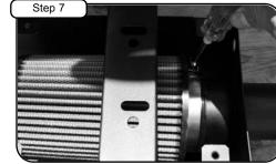
Install filter into housing and tighten clamp.
