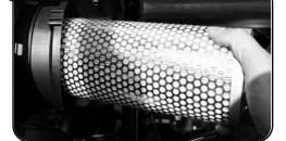
Un-clip housing cover and remove air filter.
