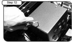
Secure cover to housing using M6 allen head bolts.
