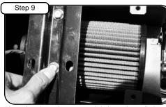
Mount housing using two stock bolts and supplied nuts and washers (tighten)
