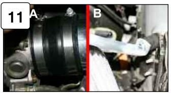
A)Install into vehicle and position coupler to throttle body and tab to isolation mount. B)Secure tab using flat washer, wavy washer and nut provided. Tighten using 10mm socket or wrench. Tighten clamps using 5/16" nut driver.
