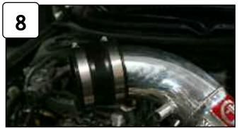
Attach coupler with clamps to tube. Do not tighten.
