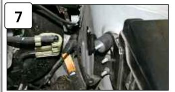
Install M6 male/female isolation mount to ECU harness bracket and secure.
