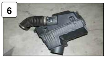
Remove stock intake out of vehicle.
