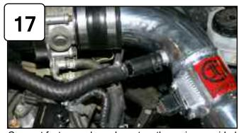
Connect factory and new hose together using provided 5/8" barb fitting. Re-connect battery terminals. Reinstall engine cover.
