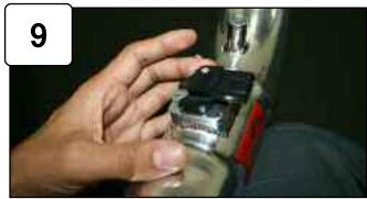
Remove MAF sensor from stock intake. Install into new intake tube and secure using provided M4 screws.
