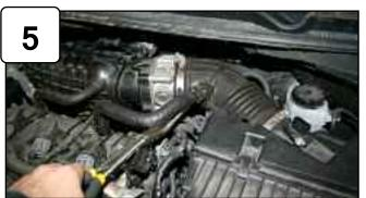
Remove crank case line from intake tube using pliers.
