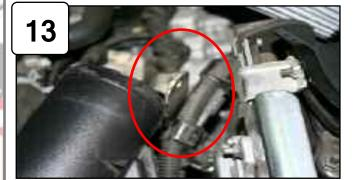
Now Install bracket and secure with screw from step 12 and tighten.
