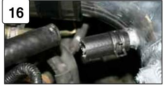
Install 5/8" hose provided to intake tube with factory clamp.
