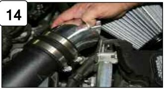
Install cold air duct using coupler with clamps provided. Using screw, nut and washer provided, tighten tab on duct to bracket using 10mm socket or wrench. Tighten clamps using 5/16" nut driver.
