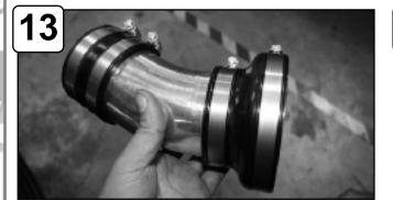
Attach couplers with clamps to intake tube.
