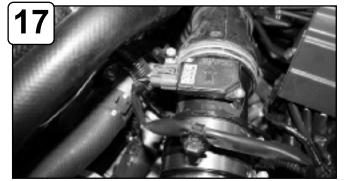
Re-connect MAF sensor harness. Tighten intake clamp using 10mm socket or wrench.
