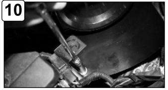
With provided washer and screw tighten down housing using 10mm socket or wrench.
