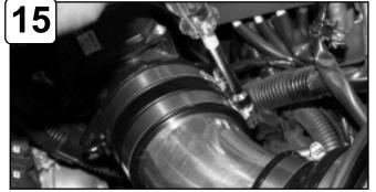
Tighten clamps using 5/16" nut driver.
