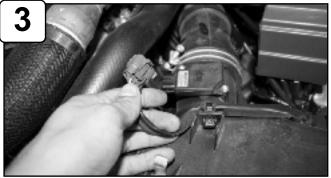
Disconnect MAF sensor harness. Loosen clamp using 10mm socket or wrench.
