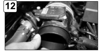
Install MAF sensor back to intake tube.
