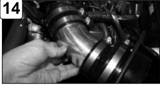
Install and position intake tube assembly to MAF sensor and adaptor.
