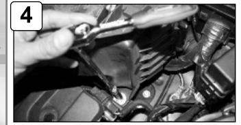
With 10mm socket or wrench loosen the bolt holding bottom half of air box.
