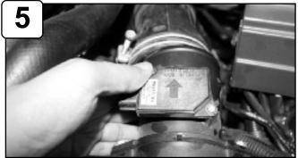
Pull back MAF sensor from intake tube.
