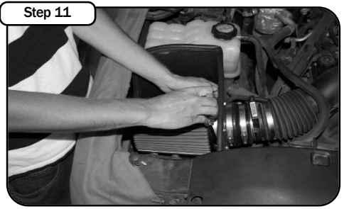
Step 11 Install intake filter into housing. Re-connect the MAF sensor. Your Stage 1 installation is now complete. Make sure you tighten all clamps and check all electrical connections. Re-check periodically. Continue onto steps 11-13 to install Stage 2.
