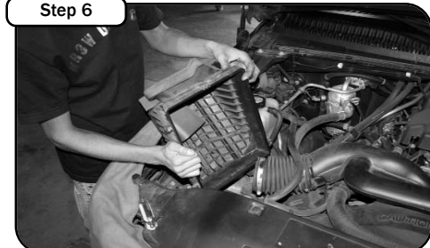
Step 6 Grab the lower portion of the airbox then lift up and out. The box is secured with rubber gromets.
