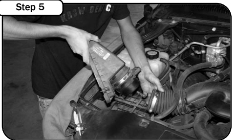
Step 5 Loosen the hose clamp connecting the MAF sensor to the airbox. Remove upper portion of the airbox and MAF Sensor. Carefully set MAF sensor to the side for later use.
