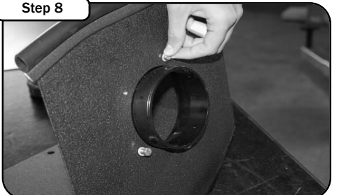
Step 8 Place the air filter adaptor inside the housing. Secure the adaptor with the M6 button head screws and M6 wavy washers provided.
