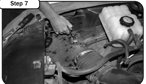
Step 7 Remove the four 10mm bolts that secure the airbox base to the chassis. Save bolts for later use. Remove airbox tray out of vehicle.
