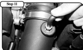
Push the breather tube onto the brass nipple. The special fitting does not require a clamp.
