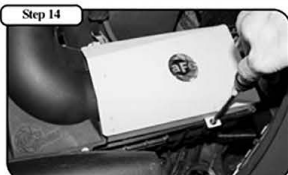
Secure the cover to the housing by tightening two of the stock screws using a phillips screwdriver. Use one of the screws provided for the tab that sits on the intake tube.
