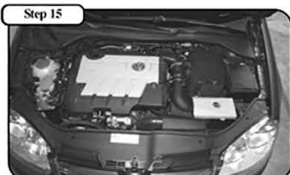
Your Stage 1 Intake is now complete. Make sure to tighten all clamps and check all electrical connections. Re-tighten clamps after a few hours of Operation. Thank you for choosing afE Power!
