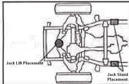
5. Once both sides are safely on jack stands, use the 3/4in deep socket and impact gun to remove the lug nuts and wheels.
