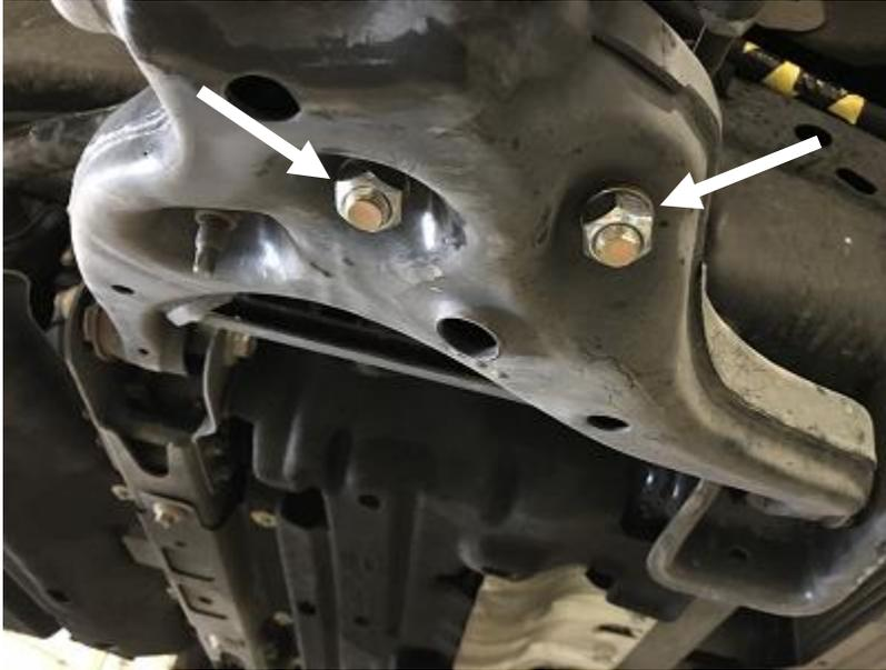
15. Use the ball joint remover to remove the upper spindle ball joint and slightly lower the jack to allow the arm to droop.
