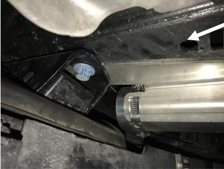
18. Place the reservoir in the bracket and tighten the hose clamps. Hose clamps should be placed through the openings in the bracket.
