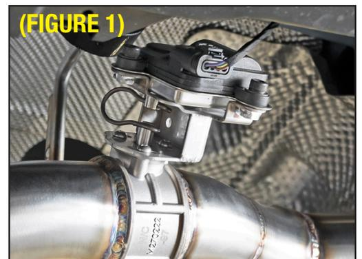
**NOTES:** aFe recommends that the tailpipe be at least 1/2"-1" away from any body panels to avoid heat related body damage. **Tighten and secure.**
