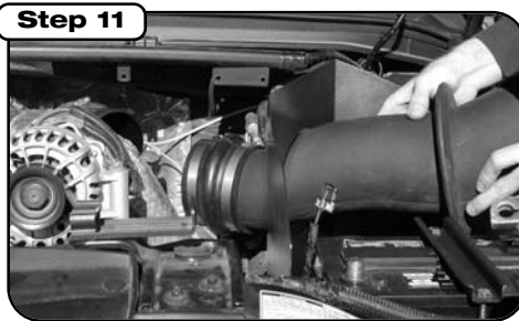
Attach coupler to intake tube and insert tube through housing. Rotate tube to line up flange holes with holes on housing. Using supplied hardware, fasten securely and tighten clamp on engine side of intake tube.
