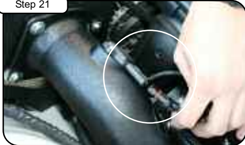
Re-connect MAF sensor harness. Re-connect battery.
