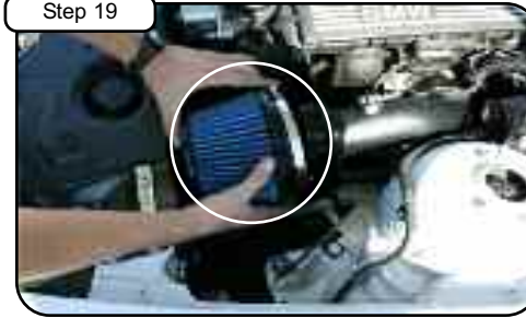
Install air filter on tube and tighten using 5/16" nut driver.
