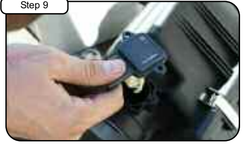
Step 9 Carefully remove MAF sensor.
