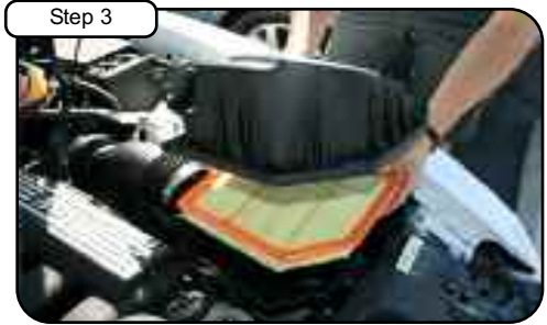
Step 3 Lift up and pull upper half of air box out. Remove air filter.
