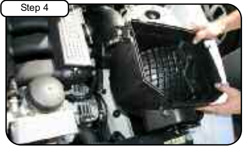
Step 4 Lift and pull bottom half of air box out of vehicle.
