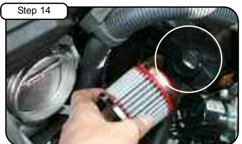
Step 14 Attach crankcase filter to smog pump and tighten using 5/16" nut driver.
