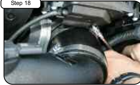
Tighten all clamps using 5/16" nut driver.
