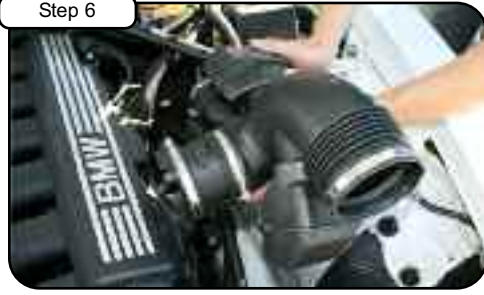
Step 6 Remove Intake tube out of vehicle.
