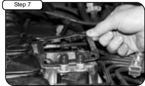
Step 7 Remove both top and bottom stock gaskets away from air grid heater. Replace with new gaskets provided. (May require a scraper or scotch brite to clean sealing surfaces.)
