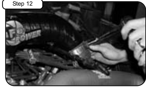
Step 12 Torque coupler hose clamp with 7/16" deep socket to 71 in. lbs.. Torque the four mounting screws from Step 11 to 18 ft. lbs..
