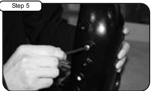
Step 5 Apply threadlocker to 1/8" NPT plugs. Install to aFe manifold using 3/16" allen key.
