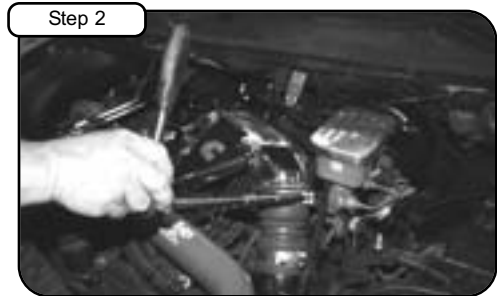
Step 2 Use 7/16" deep socket with ratchet to loosen the intercooler coupler hose clamp. Remove the screw holding engine oil dipstick.
