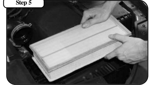
Remove the stock air filter and plastic grill from the factory air box.
