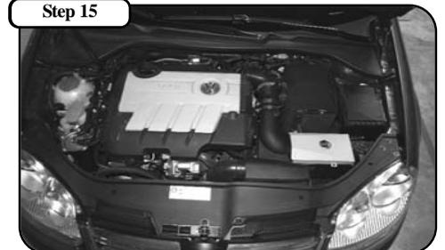
**Your Stage 1 Intake is now complete.** Make sure to tighten all clamps and check all electrical connections. Re-tighten clamps after a few hours of Operation. Thank you for choosing aFePower!
