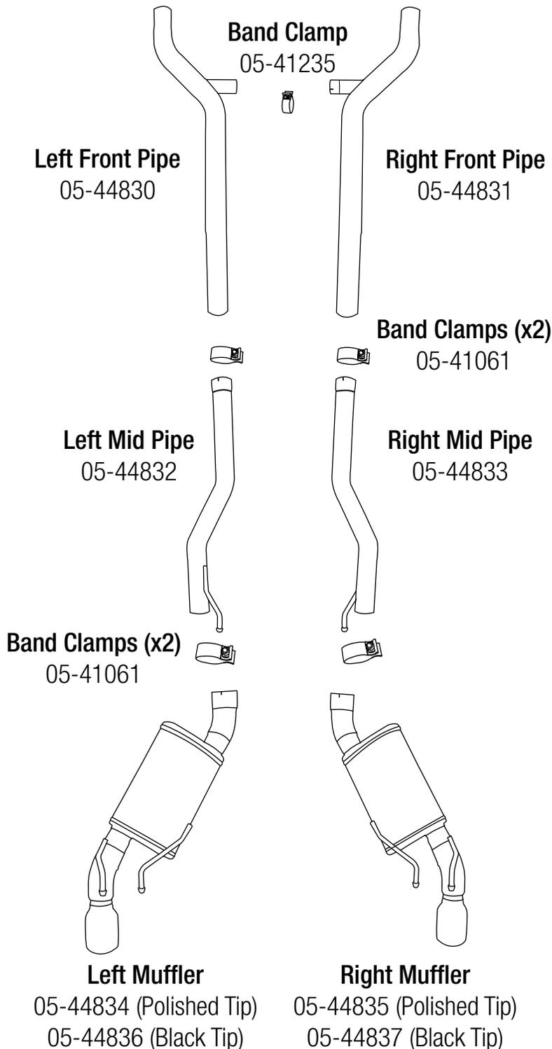
**Caution:** Allow time for your vehicle to cool down prior to installation. When working on or under your vehicle proceed with caution. Exhaust systems reach high temperatures and may cause serious burns. Wear protective safety equipment; eye goggles and gloves to ensure a safe installation.
